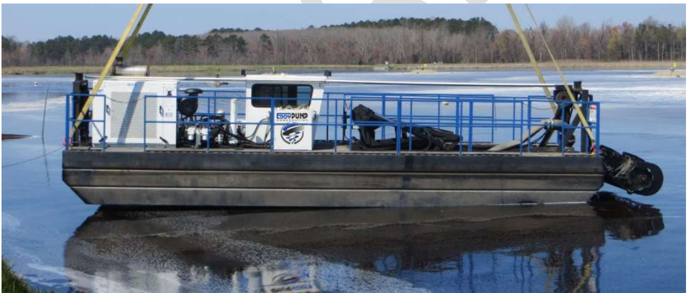
Figure 18 Example Floating Dredge System Suitable for Mixing RORW and Bauxite Residuals
