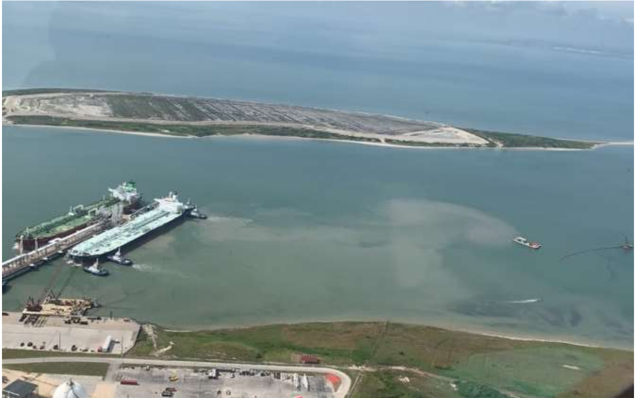
Photo showing a sediment plume from docking vessels at Moda's existing pier and the close proximity and impact of the sediment plume on the existing seagrasses and wetland areas. August 2020.
