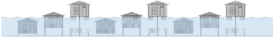
Figure 15. Buoyant foundations (Buoyant Foundation Project, 2020)
