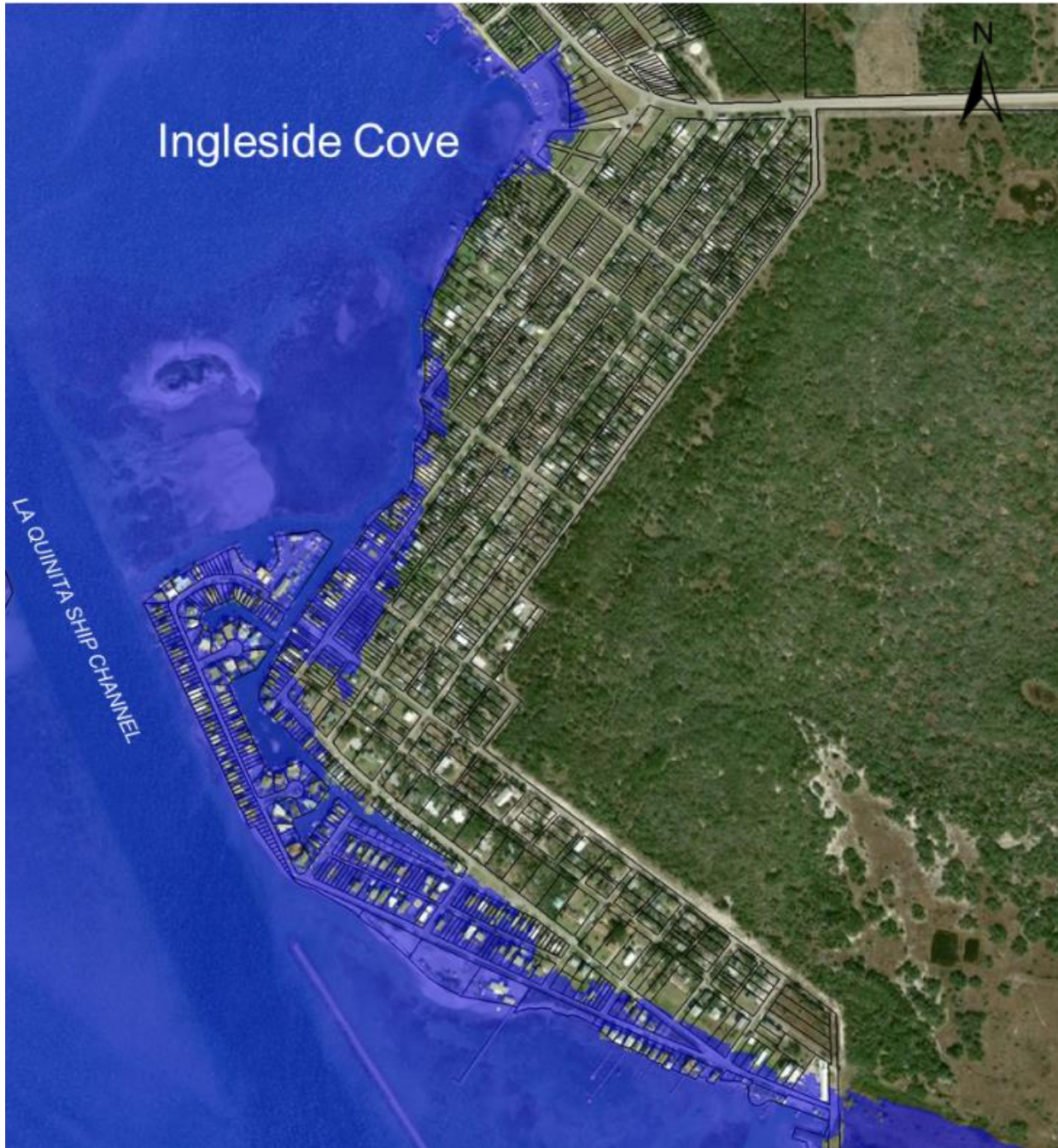
Figure 8. Map representing flood coverage in blue for the 2080 1-year flood event (+5.5 ft NAVD88)
