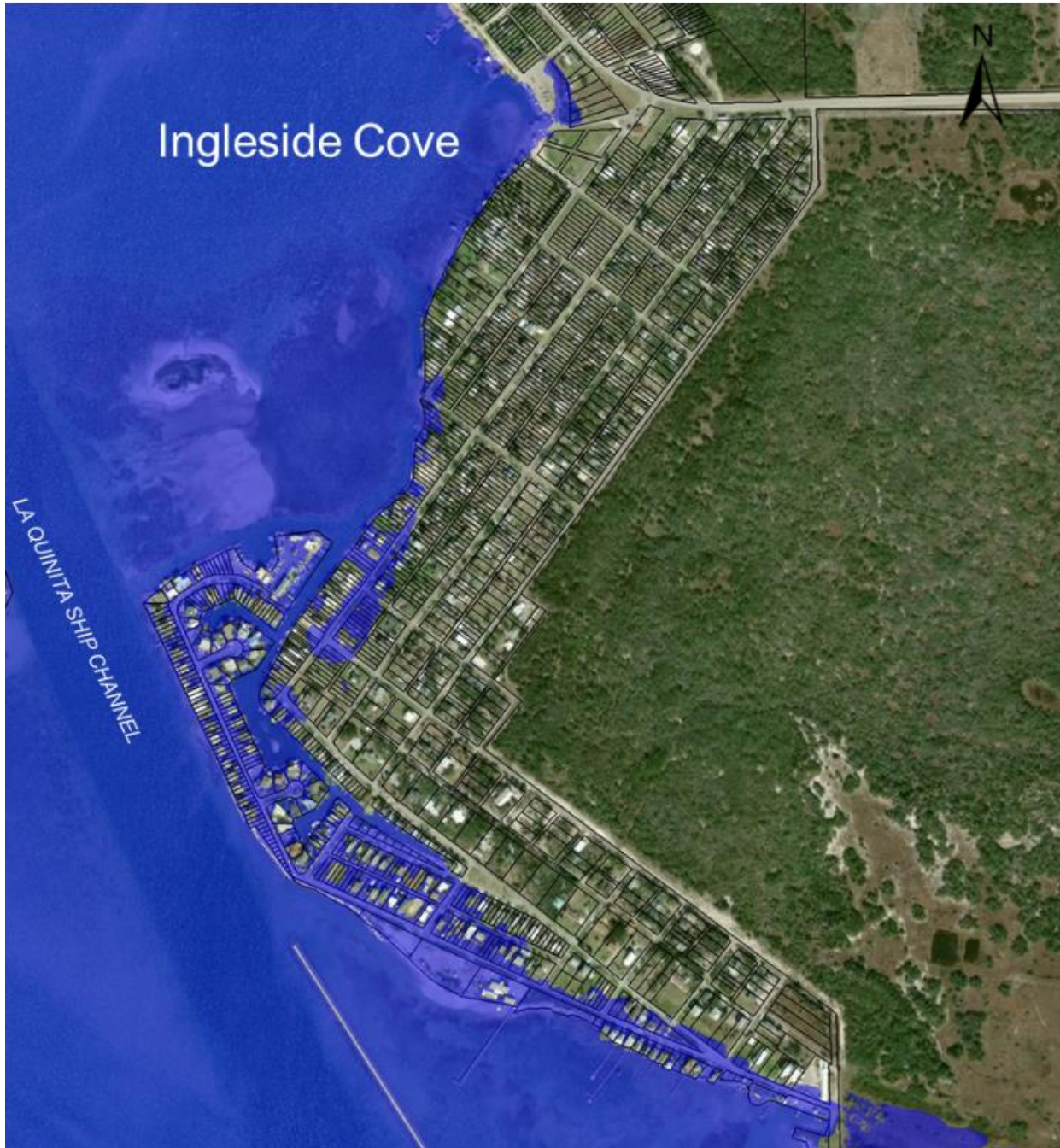
Figure 6. Map representing flood coverage in blue for the 2040 1-year flood event (+3.9 ft NAVD88)
