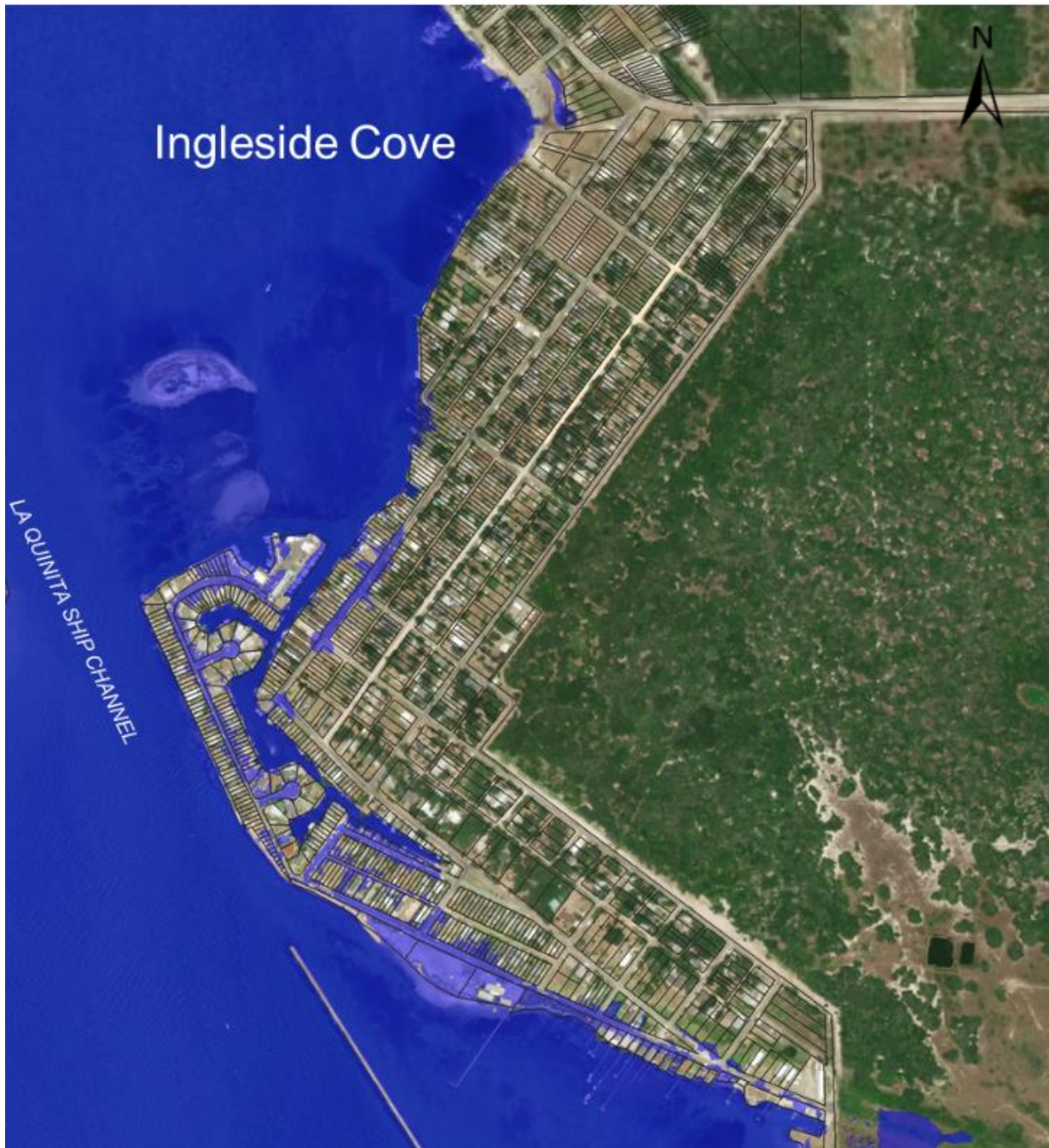
Figure 5. Map representing flood coverage in blue for the present-day 1-year event (2.9 ft NAVD88)
