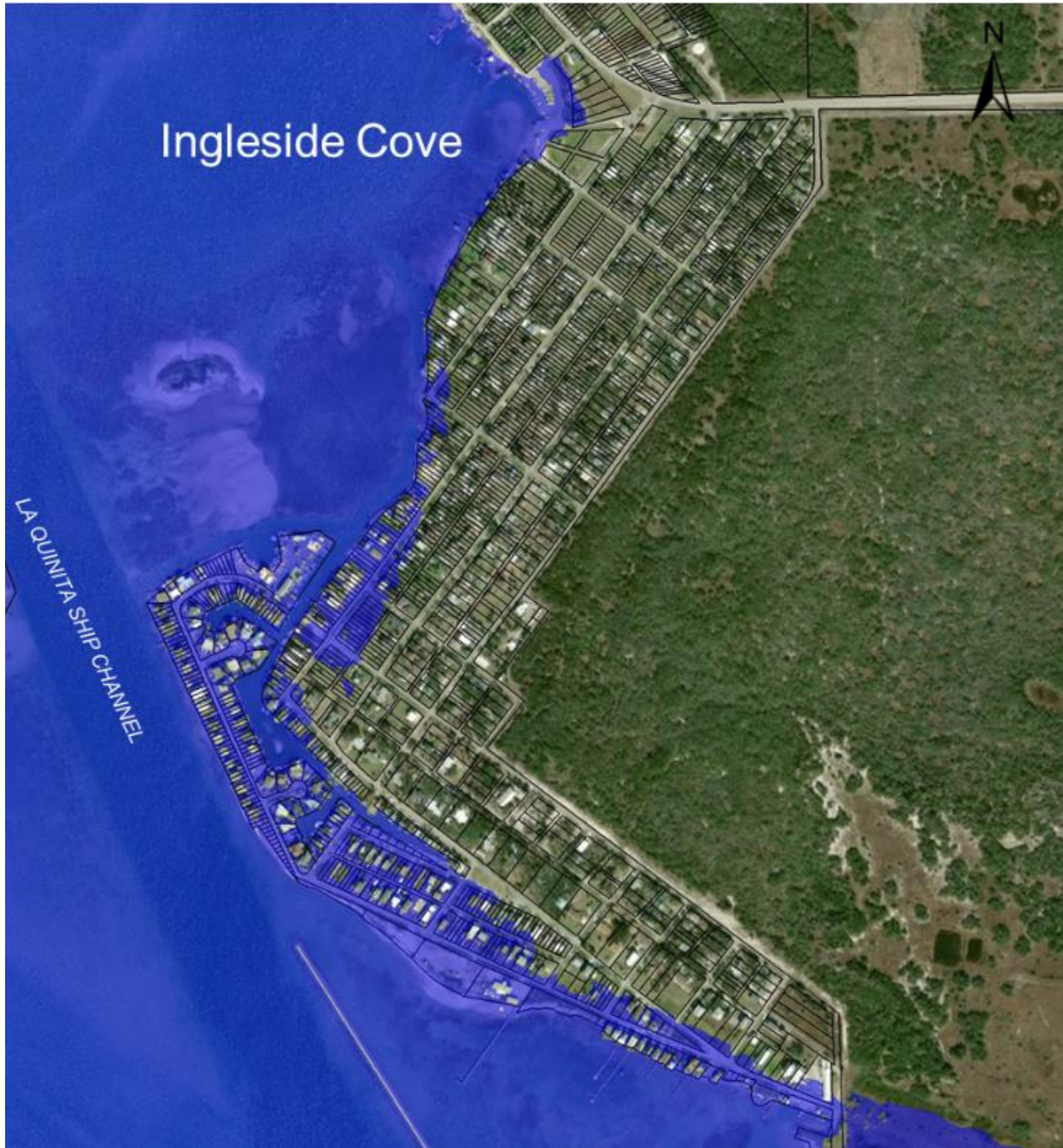
Figure 7. Map representing flood coverage in blue for the 2060 1-year flood event (+4.5 ft NAVD88)
